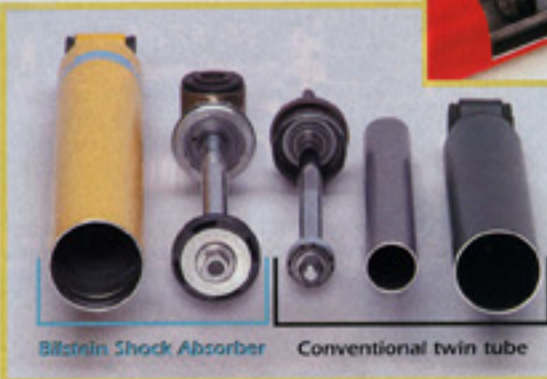
The Bilstein Gas Pressure Shock Absorber's monotube design (left) allows excessive heat to dissipate more efficiently, eliminating fade and prolonging shock life over a conventional twin tube shock (right).
