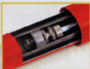
Conventional twin tube shocks trap heat.
